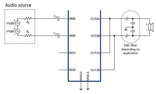
Figure 9-5 Parallel Bridge Tied Load (PBTL) configuration
