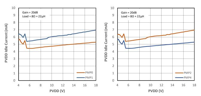
Figure 11-19 PVDD Idle Current vs PVDD for PMP0 & PMP1
