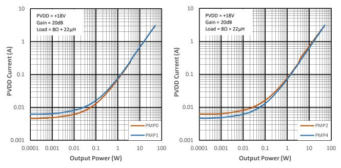
Figure 11-17 PVDD Current vs Output Power for PMP0 & PMP1
