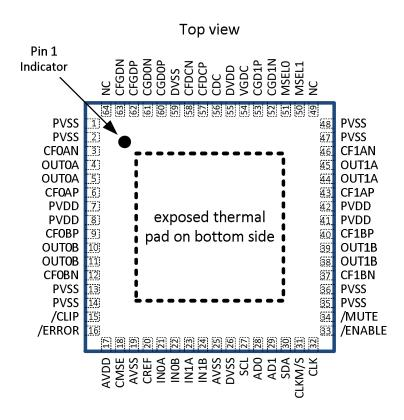
Figure 4-1 Pinout MA12040QFN
