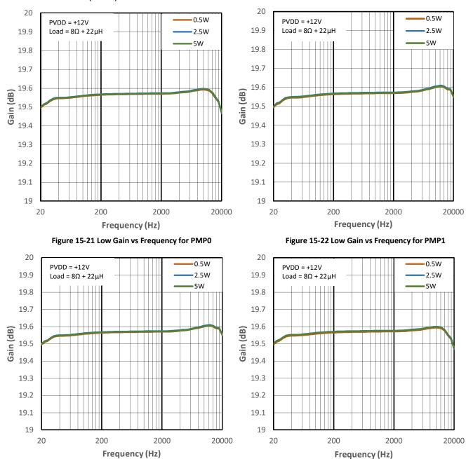
Figure 15-23 Low Gain vs Frequency for PMP2
