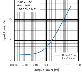
Figure 14-15 Input Power vs Output Power for PMP2
