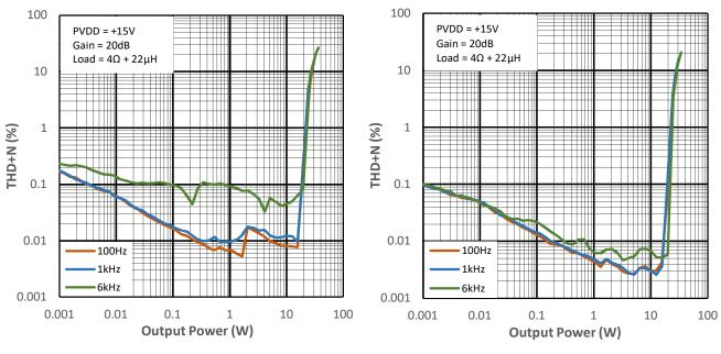
Figure 12-1 THD+N vs Output Power for PMP0
