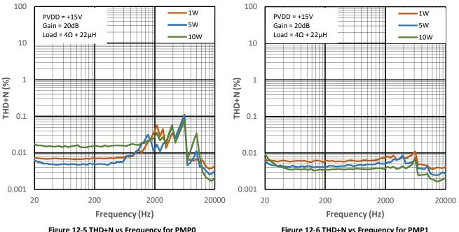
Figure 12-5 THD+N vs Frequency for PMP0
