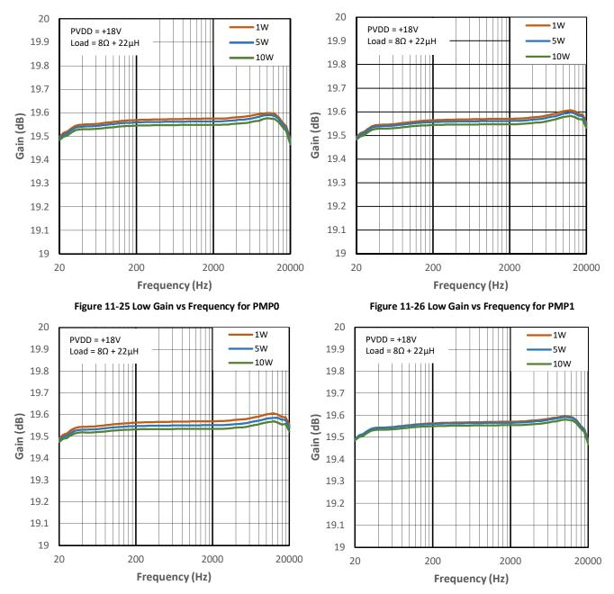
Figure 11-27 Low Gain vs Frequency for PMP2
