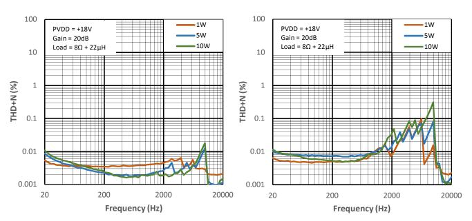
Figure 11-7 THD+N vs Frequency for PMP2
