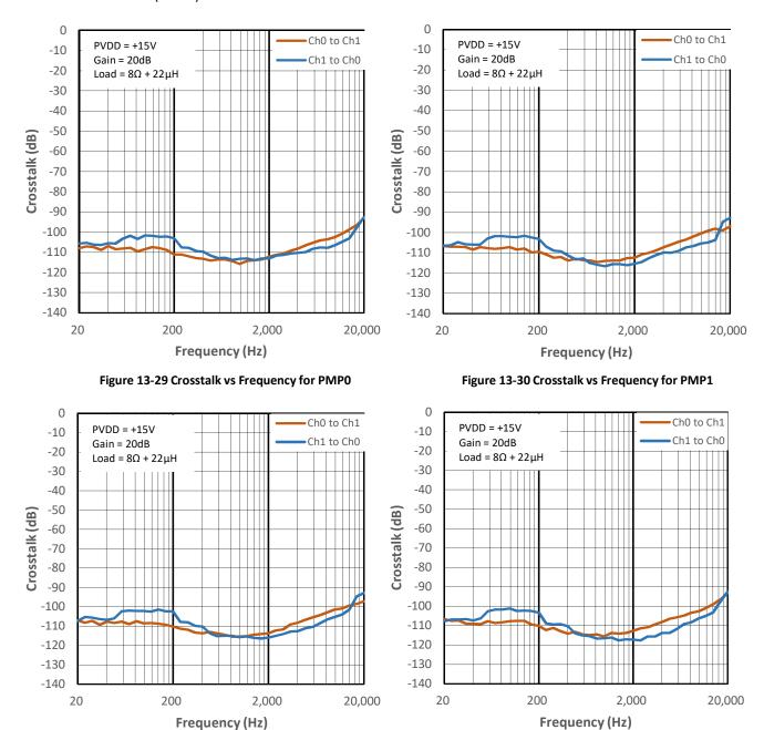
Figure 13-35 Crosstalk vs Frequency for PMP2
