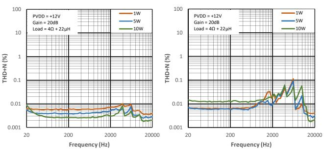
Figure 14-7 THD+N vs Frequency for PMP2
