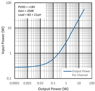
Figure 11-13 Input Power vs Output Power for PMP0
