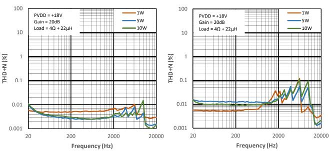
Figure 10-7 THD+N vs Frequency for PMP2
