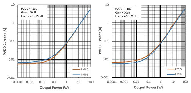
Figure 10-17 PVDD Current vs Output Power for PMP0 & PMP1
