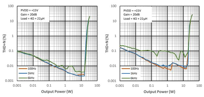
Figure 12-3 THD+N vs Output Power for PMP2
