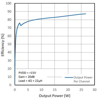
Figure 12-9 PMP0 Efficiency (VDD+PVDD) vs Output Power
