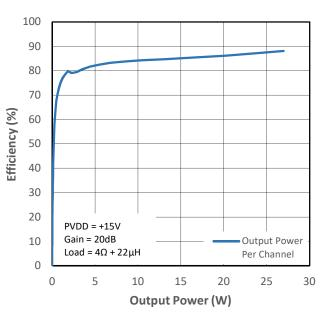
Figure 12-12 PMP4 Efficiency (VDD+PVDD) vs Output Power
