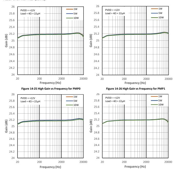
Figure 14-27 High Gain vs Frequency for PMP2
