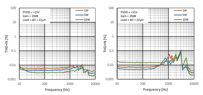
Figure 12-7 THD+N vs Frequency for PMP2
