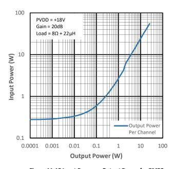
Figure 11-15 Input Power vs Output Power for PMP2
