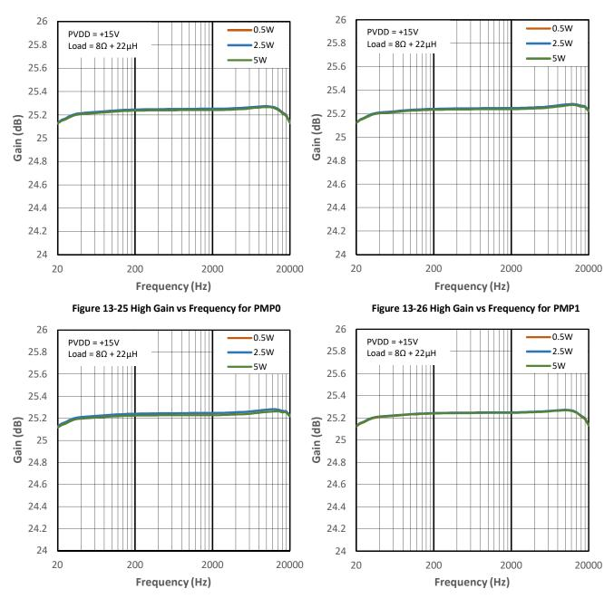
Figure 13-27 High Gain vs Frequency for PMP2
