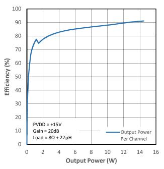
Figure 13-9 PMP0 Efficiency (VDD+PVDD) vs Output Power
