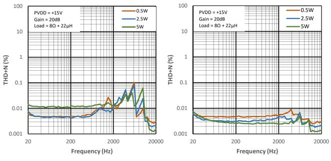
Figure 13-5 THD+N vs Frequency for PMP0
