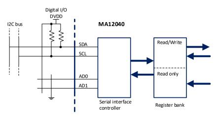
Figure 8-2. I2C bus interface and register bank
