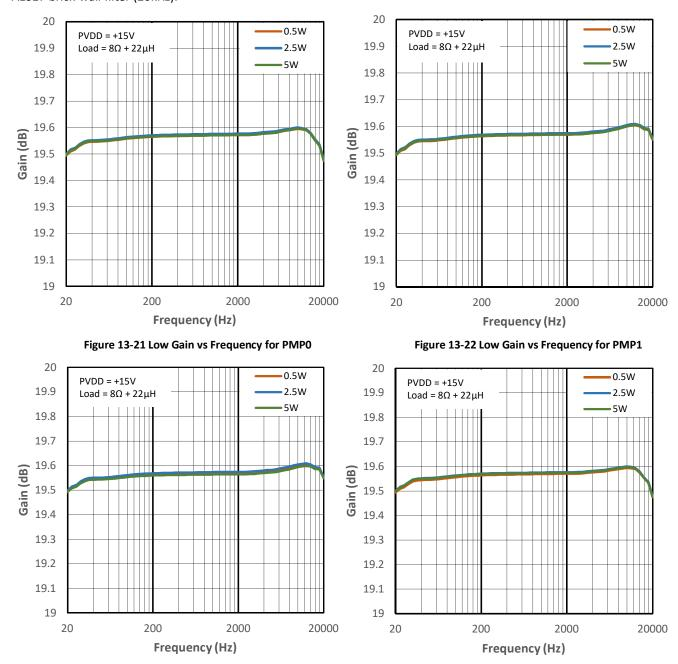
Figure 13-23 Low Gain vs Frequency for PMP2
