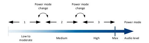
Figure 8-1 Illustration of automatic power mode selection ranges
