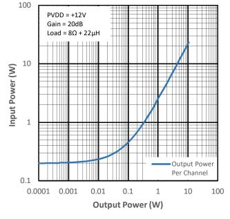
Figure 15-15 Input Power vs Output Power for PMP2
