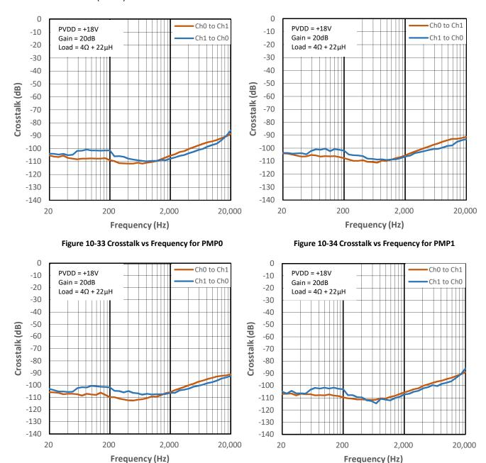
Figure 10-35 Crosstalk vs Frequency for PMP2
