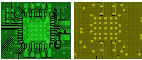
Figure 9-6 Example of 2-layer PCB layout, top and bottom layers
