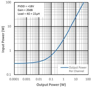
Figure 10-13 Input Power vs Output Power for PMP0
