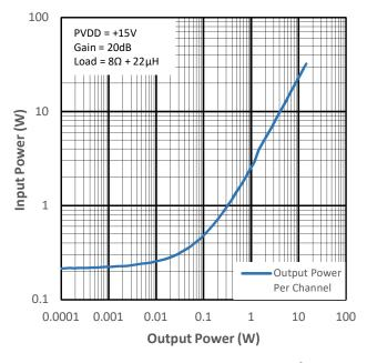
100 PVDD = +15V Gain = 20dB Load =  $8\Omega + 22\mu H$ 10 Input Power (W) **Output Power** Per Channel 0.1 0.0001 0.001 0.01 0.1 10 100 **Output Power (W)**
