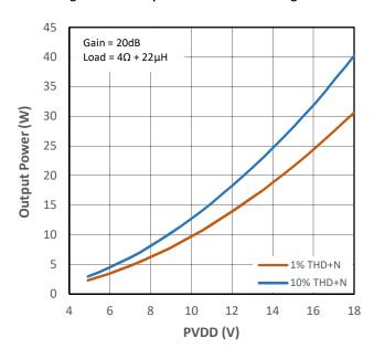
Figure 10-23 Output Power vs PVDD Voltage for PMP2
