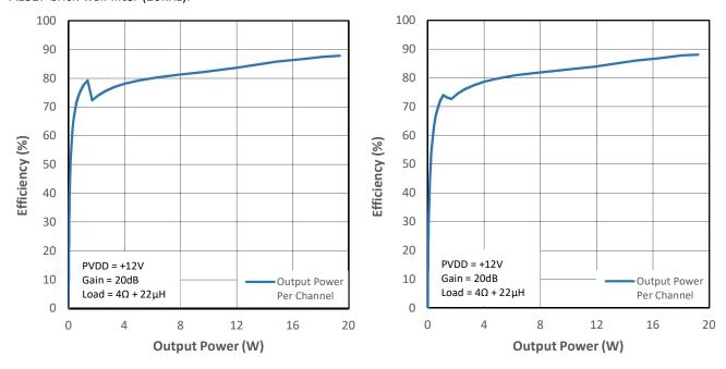
Figure 14-9 PMP0 Efficiency (VDD+PVDD) vs Output Power
