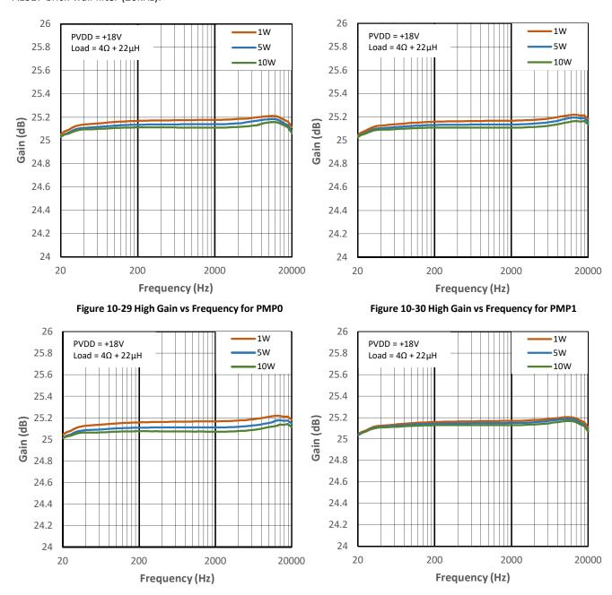
Figure 10-31 High Gain vs Frequency for PMP2
