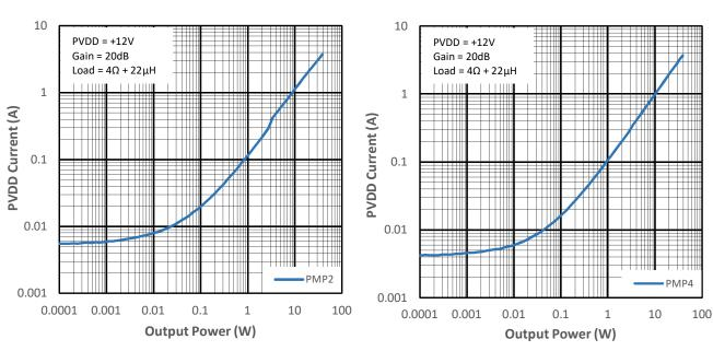
Figure 14-19 PVDD Current vs Output Power for PMP2
