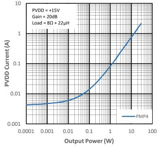
Figure 13-19 PVDD Current vs Output Power for PMP2
