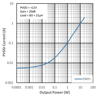
Figure 15-17 PVDD Current vs Output Power for PMP0
