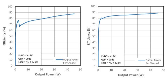
Figure 10-11 PMP2 Efficiency (VDD+PVDD) vs Output Power
