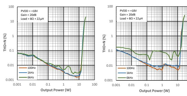
Figure 11-3 THD+N vs. Output Power for PMP2
