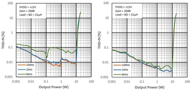
Figure 13-1 THD+N vs. Output Power for PMP0
