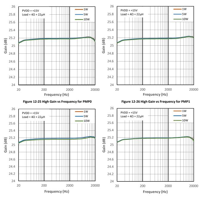
Figure 12-27 High Gain vs Frequency for PMP2
