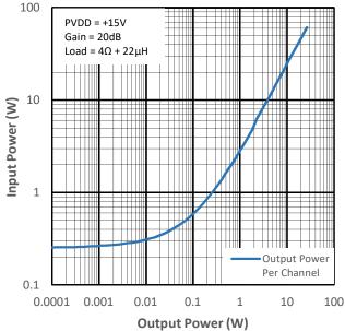
Figure 12-13 Input Power vs Output Power for PMP0
