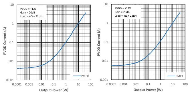
Figure 14-17 PVDD Current vs Output Power for PMP0
