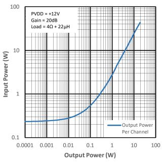
Figure 14-13 Input Power vs Output Power for PMP0
