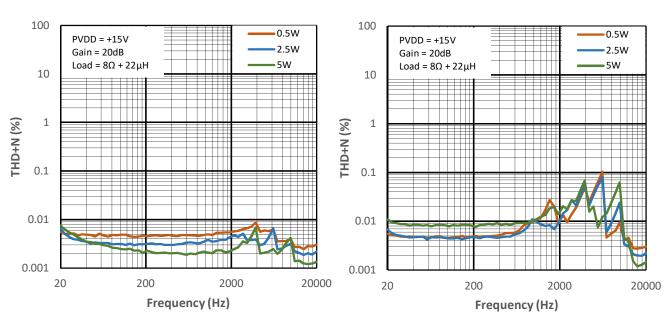
Figure 13-7 THD+N vs Frequency for PMP2
