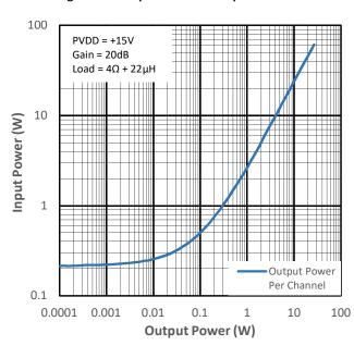
Figure 12-16 Input Power vs Output Power for PMP4
