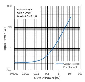
Figure 13-16 Input Power vs Output Power for PMP4
