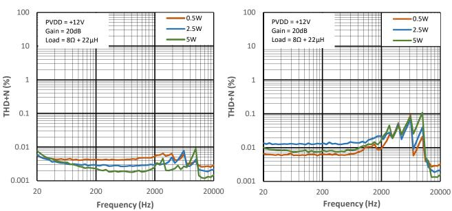
Figure 15-7 THD+N vs Frequency for PMP2
