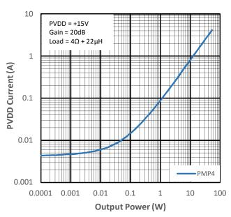
Figure 12-19 PVDD Current vs Output Power for PMP2
