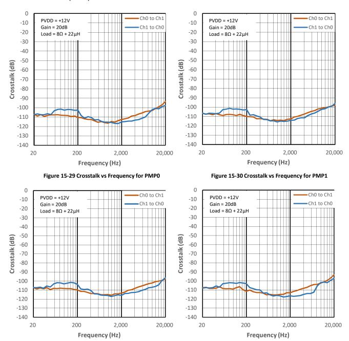
Figure 15-35 Crosstalk vs Frequency for PMP2
