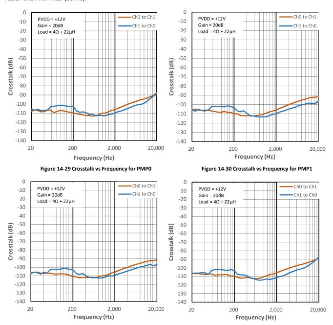
Figure 14-31 Crosstalk vs Frequency for PMP2
