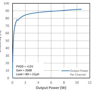
Figure 15-12 PMP4 Efficiency (VDD+PVDD) vs Output Power
