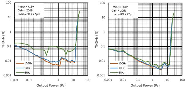
Figure 11-1 THD+N vs. Output Power for PMP0
