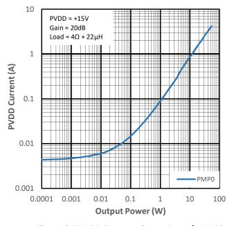
10 PVDD = +15V Gain = 20dB Load =  $4\Omega + 22\mu H$ 1 PVDD Current (A) 0.1 0.01 0.001 100 0.0001 0.001 0.01 0.1 10 **Output Power (W)**
