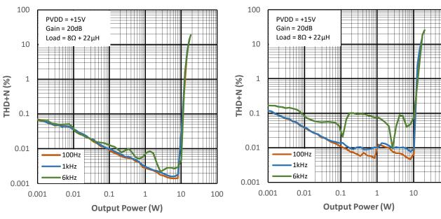
Figure 13-3 THD+N vs. Output Power for PMP2
