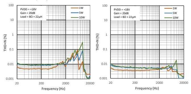
Figure 11-5 THD+N vs Frequency for PMP0
