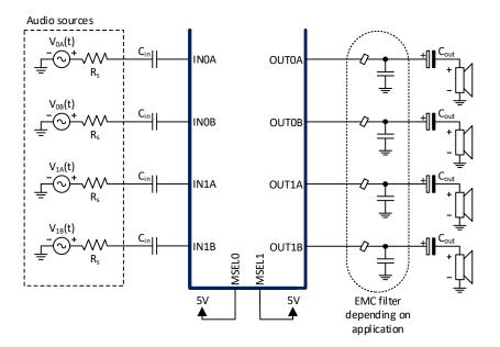
Figure 9-3 Four channel, single ended (SE) configuration
