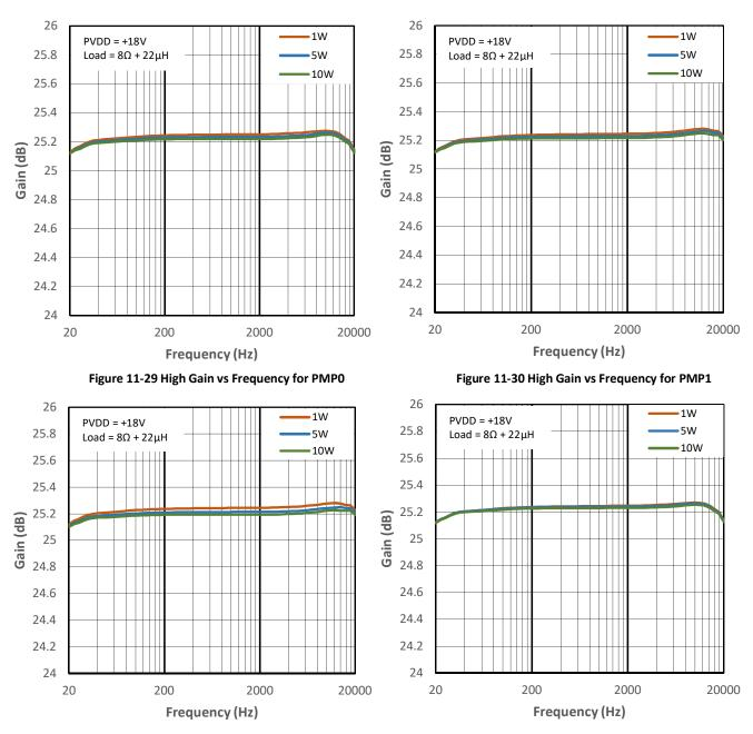
Figure 11-31 High Gain vs Frequency for PMP2
