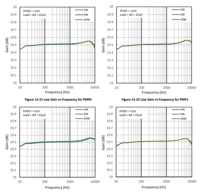
Figure 12-23 Low Gain vs Frequency for PMP2
