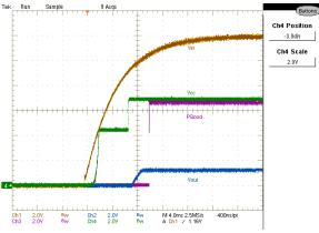
Figure 32: Startup with full load, VCC signal CH1:Vin, CH2:Vout, CH3:PGood, CH4:VCC
