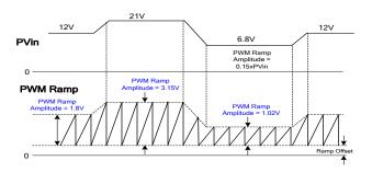
Figure 13: Timing Diagram for Feed-Forward (F.F.) Function
