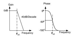
Figure 25: Gain and Phase of LC filter
