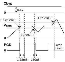
Figure 19: PGood Timing Diagram
