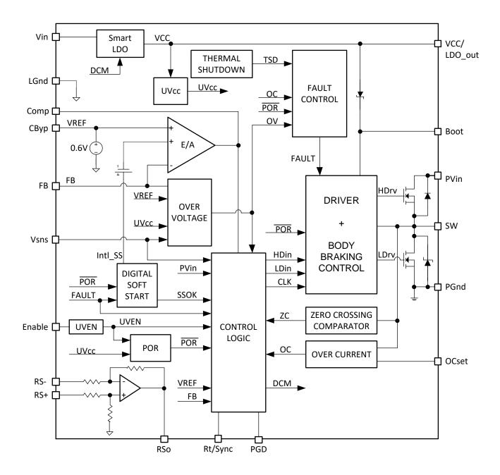
Figure 3: IR3447 Simplified Block Diagram
