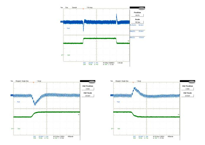
Figure 38: Vout Transient Response, 17.5A to 25A step at 2.5A/uSec CH2:Vout, CH4:Iout (10A/V)
