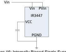
Figure 16: Internally Biased Single Supply Configuration
