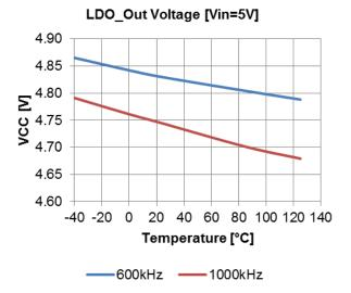
Figure 18: LDO\_Out Voltage in dropout mode
