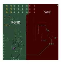
Figure 42d: IRDC3447 Demo board Layout Considerations - Mid Layer 2
