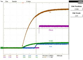
Figure 31: Startup with full load, Enable Signal CH1:Vin, CH2:Vout, CH3:PGood, CH4:Enable
