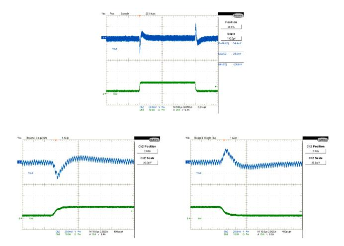
Figure 37: Vout Transient Response, 2.5A to 10.0A step at 2.5A/uSec CH2:Vout, CH4:lout (10A/V)
