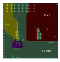
Figure 42b: IRDC3447 Demo board Layout Considerations - Bottom Layer
