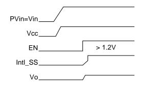
Figure 5: Recommended startup for Normal operation
