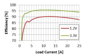
Figure 2: Efficiency [Vin=12V, Fsw=600kHz]
