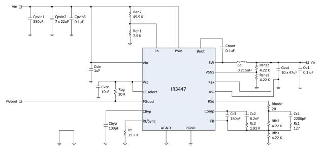
Figure 28: Application circuit for a 12V to 1.2V, 25A Point of Load Converter Using the Internal LDO
