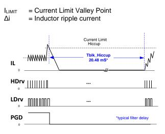
Figure 9: Timing Diagram for Current Limit Hiccup
