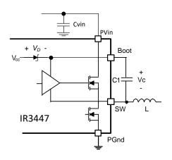
Figure 24: Bootstrap circuit to generate Vc voltage
