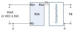
Figure 11: Remote Sense Configuration for Vout less than VCC-1.5V
