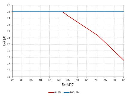
Vin=PVin=12V, Vout =5.0V, VCC=internal LDO (6.8V), Fs = 600kHz
