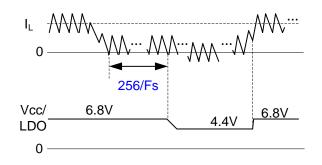
Figure 14: Time Diagram for Smart LDO
