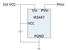
Figure 17: Externally Biased Configuration
