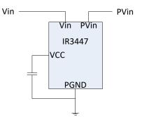
Figure 15: Internally Biased Configuration
