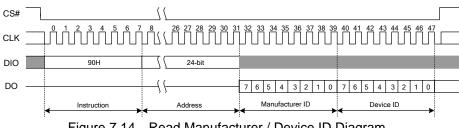
Figure 7.14 Read Manufacturer / Device ID Diagram
