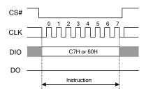
Figure 7.10 Chip Erase Instruction Sequence Diagram
