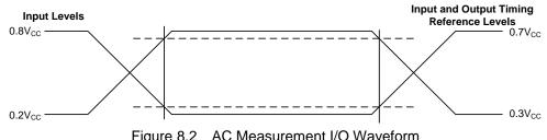
Figure 8.2 AC Measurement I/O Waveform
