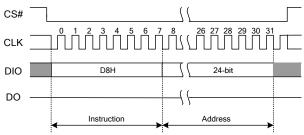
Figure 7.9 Block Erase Instruction Sequence Diagram
