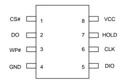
Figure 3.1 8-pin SOP (150/208mil)/ PDIP (300mil)
