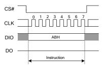
Figure 7.12 Release Power-down Instruction Sequence
