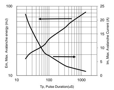
Figure 7: Single pulse Max. Avalanche Energy and Current
