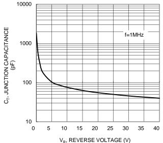
Figure 6. Typical Junction Capacitance
