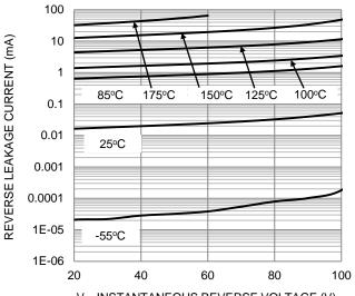
V<sub>R</sub>, INSTANTANEOUS REVERSE VOLTAGE (V) Figure 2. Typical Reverse Characteristics
