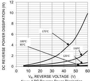
Figure 4 DC Reverse Power Dissipation
