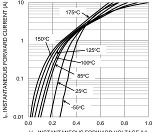
V<sub>F</sub>, INSTANTANEOUS FORWARD VOLTAGE (V) Figure 1. Typical Forward Characteristics
