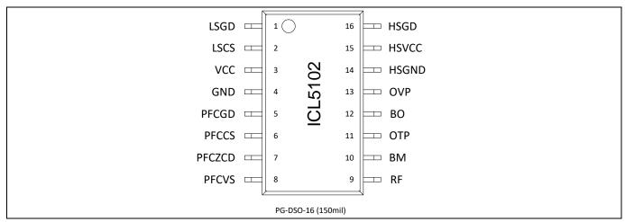
Figure 2 Pinning of ICL5102
