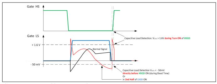
Figure 20 HB Capacitive Mode Detection
