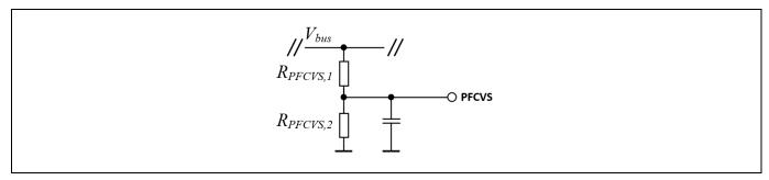
Figure 9 ICL5102 PFC Bus Voltage Sensing
