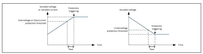
Figure 11 Excess of threshold due to Blanking Time
