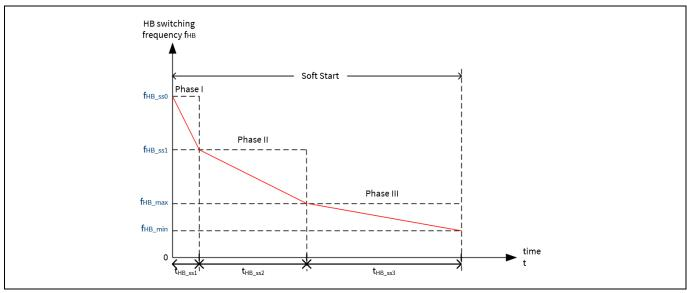
Figure 14 TCO for Half-Bridge Soft-start
