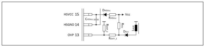
Figure 19 HB Output OVP Detection Circuit
