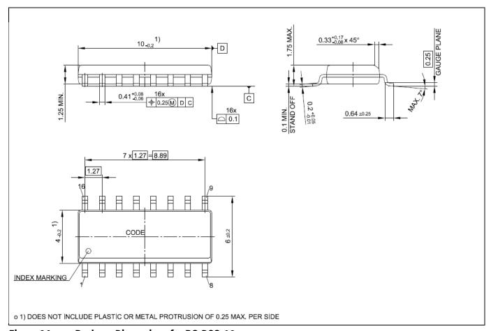
Figure 24 Package Dimensions for PG-DSO-16
