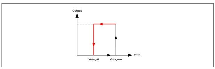
Figure 22 External Over-Temperature Protection
