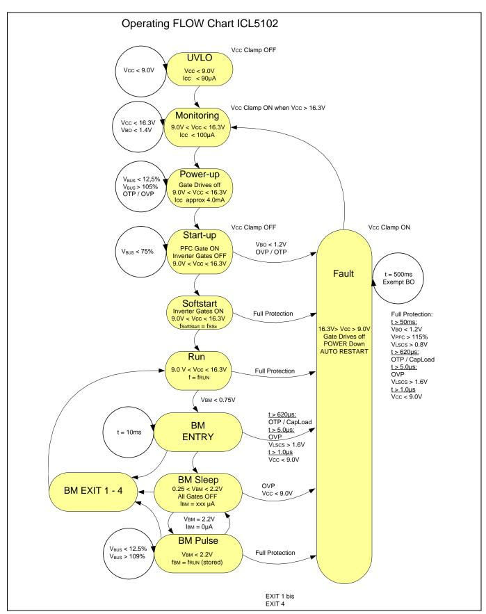
Figure 23 ICL5102 Operation Flow Chart
