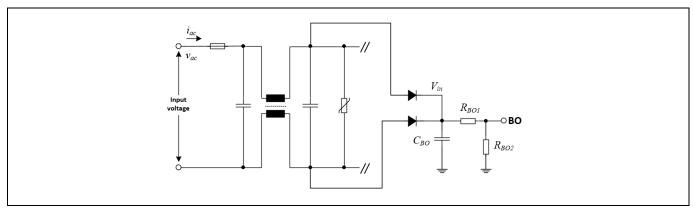
Figure 10 ICL5102 Input Voltage Sensing
