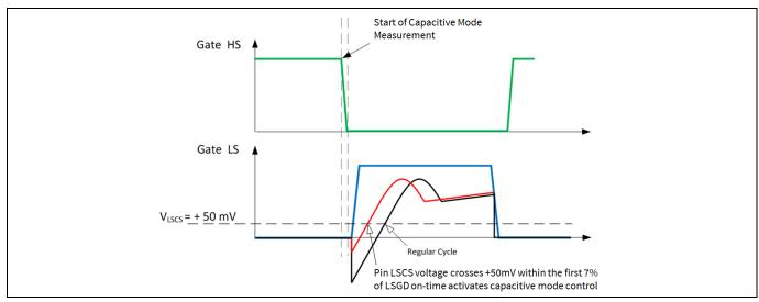
Figure 21 HB Capacitive Mode Regulation
