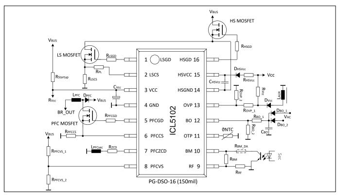
Figure 3 ICL5102 Pin Connection
