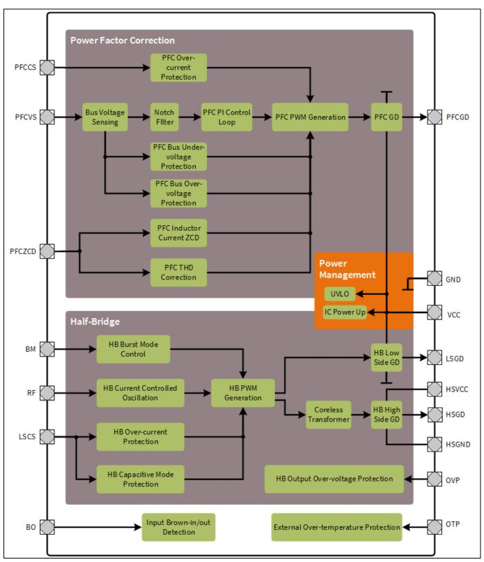
Figure 4 ICL5102 Functional Block Diagram
