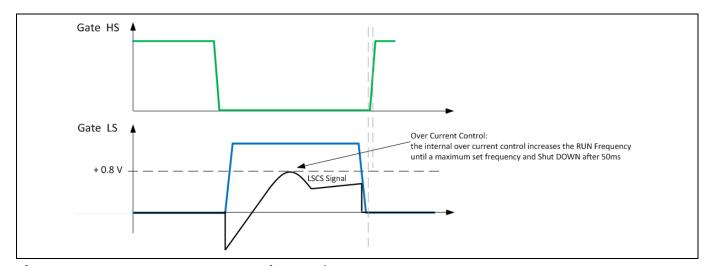
Figure 18 HB Over-current Protection Level 1
