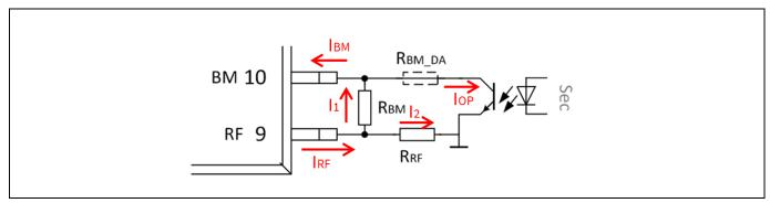
Figure 12 ICL5102 RF Pin Current Definition
