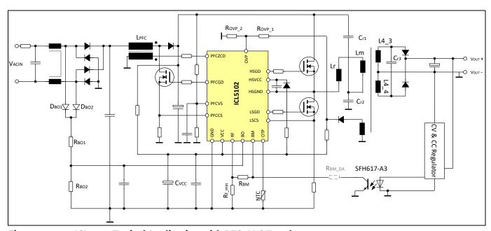
Figure 1 ICL5102 Typical Application with PFC+LLC Topology
