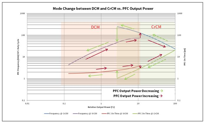
Figure 7 ICL5102 Operating Frequency and On-Time in CrCM and DCM
