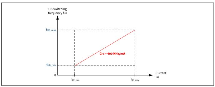
Figure 13 CCO of ICL5102 in Normal Operation
