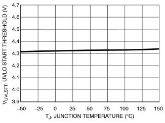
Figure 6. UVLO Start Threshold vs. Junction Temperature
