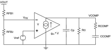
Figure 29. Feedback Compensator Network Model
