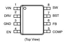
Figure 3. Pin Connections
