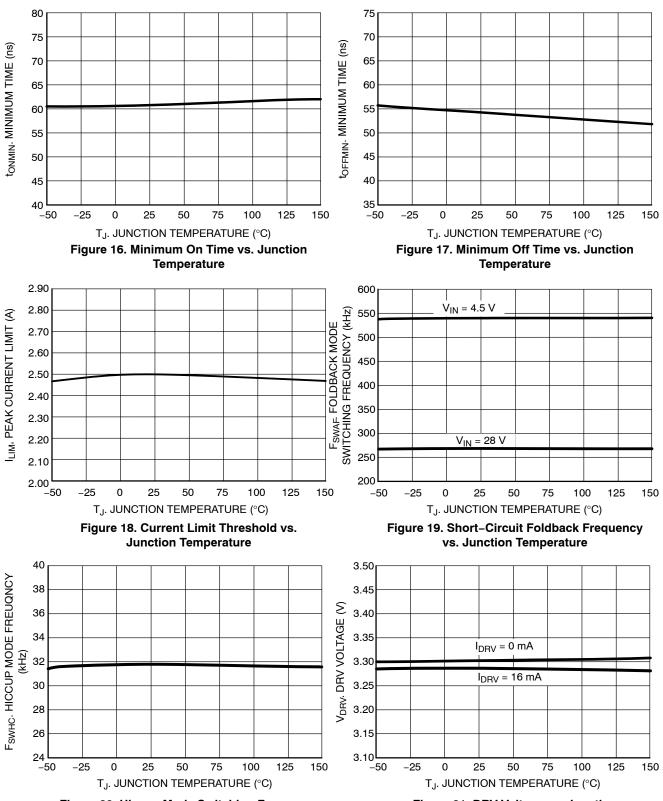
Figure 20. Hiccup Mode Switching Frequency vs. Junction Temperature
