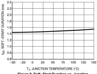
Figure 8. Soft-Start Duration vs. Junction Temperature
