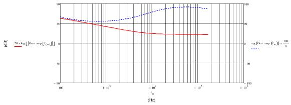
Figure 32. Bode Plot of the OTA Compensator
