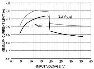
Figure 26. NCV890230 Load Current Capability with 4.7 µH Inductor
