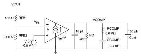
Figure 31. Example of the Feedback Compensation Network
