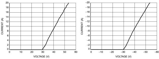
Figure 5. Pin 1 to Pin 2 TLP IV Curve
