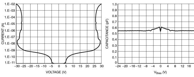
Figure 9. Typical IV Characteristics
