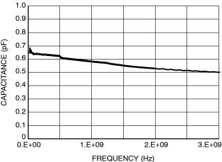
Figure 12. Typical Capacitance over Frequency
