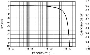
Figure 11. Typical Insertion Loss
