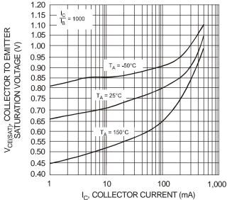
Fig. 2, Collector Emitter Saturation Voltage vs. Collector Current
