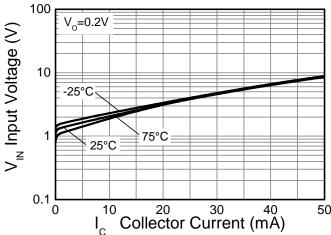
**Input Voltage v Collector Current**
