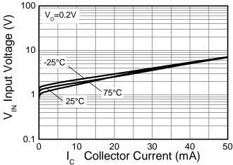
Input Voltage v Collector Current
