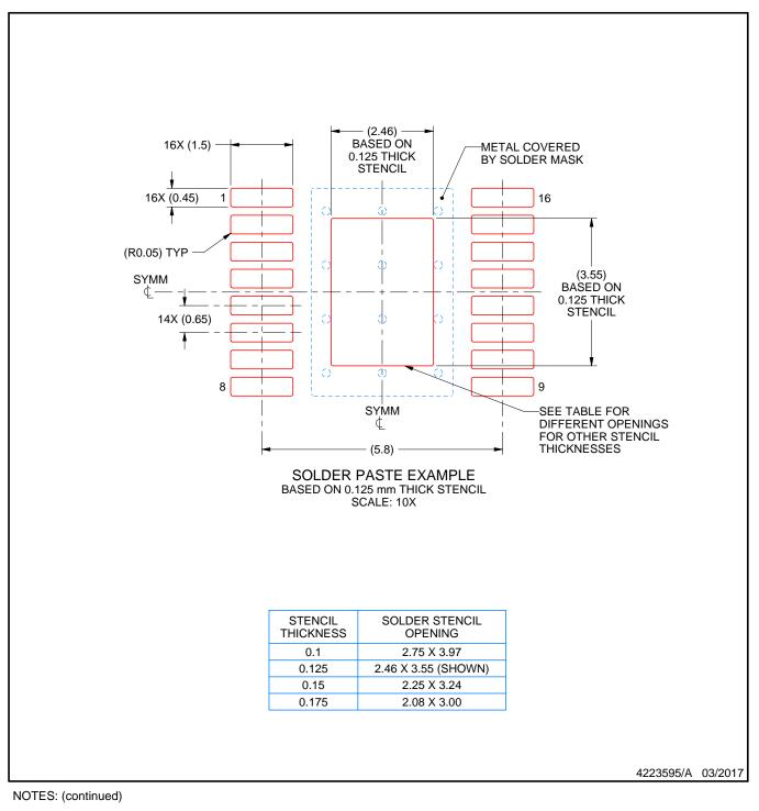
10. Laser cutting apertures with trapezoidal walls and rounded corners may offer better paste release. IPC-7525 may have alternate design recommendations.
