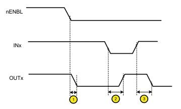
Figure 1. DRV8803 Timing Requirements
