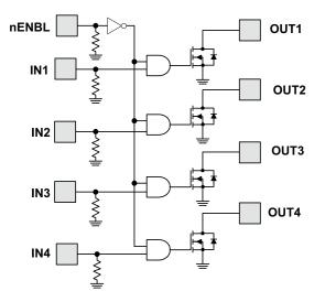
Figure 6. Parallel Interface Operation
