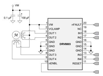
Figure 7. Typical Application Schematic
