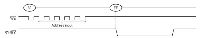
If a command other than "85h", "10h", "11h", "15h" or "FFh" is input, the Program operation is not performed and the device operation is set to the mode which the input command specifies.
