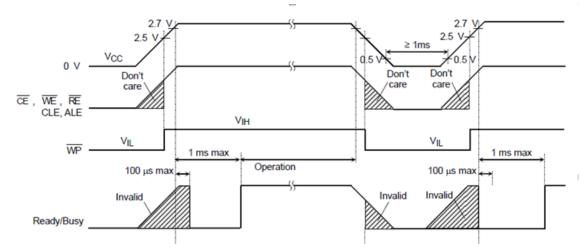
(2)Power-on Reset The following sequence is necessary because some input signals may not be stable at power-on.
