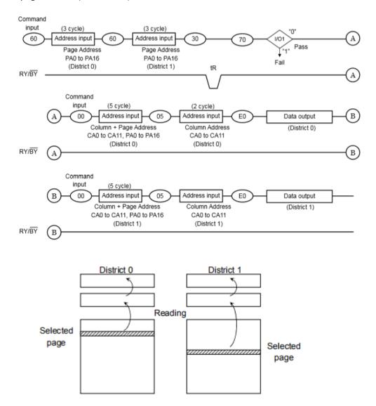
The data transfer operation from the cell array to the Data Cache via Page Buffer starts on the rising edge of  $\overline{\text{WE}}$  in the 30h command input cycle (after the 2 Districts address information has been latched). The device will be in the Busy state during this transfer period.
