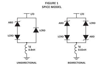
ABD - Avalanche Breakdown Diode (TVS) LCRD: Low Capacitance Rectifier Diode Lg - Lead Inductance
