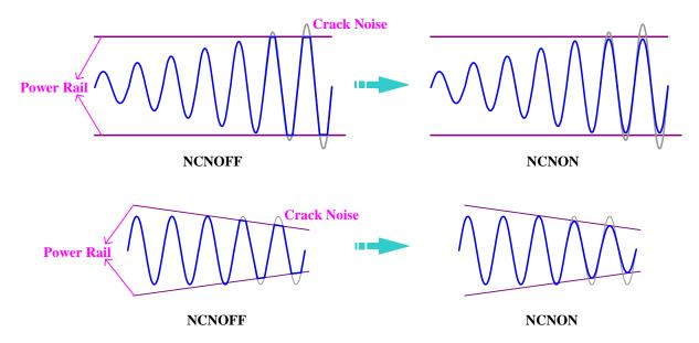
Figure 8. NCN Function Diagram
