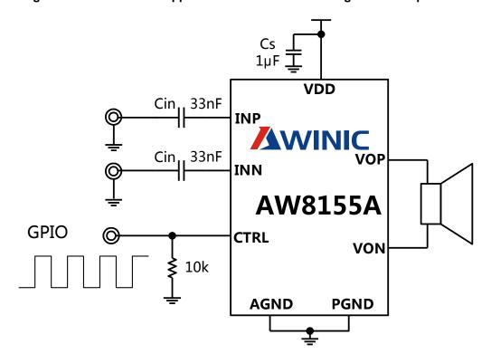
Figure 3. AW8155A Application Schematic With Differential Input
