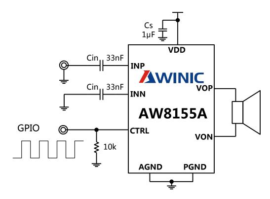
Figure 2. AW8155A Application Schematic With Single-Ended Input
