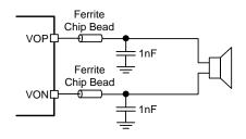
Figure 12. Ferrite Chip Bead and capacitor
