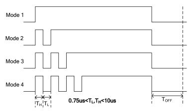
Figure 5. One-Wire pulse control
