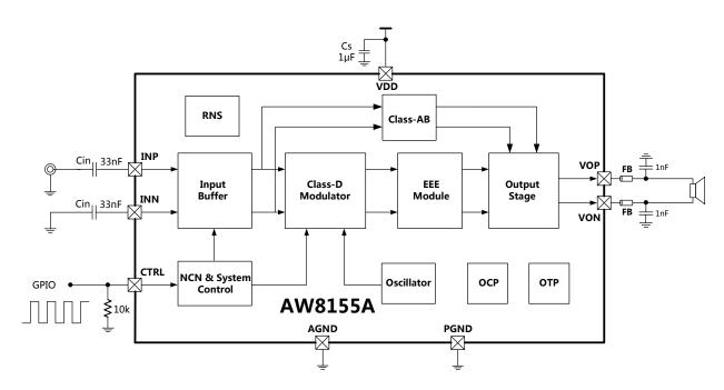
Figure 4. Functional Block Diagram of AW8155A
