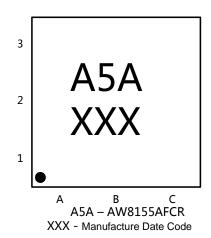
Figure 1. Pin Configuration and Top Mark of AW8155A
