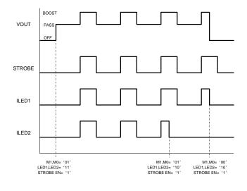
Fig 47 IR Mode with Boost
