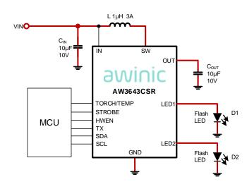
Fig 1 Typical Application Circuit of AW3643
