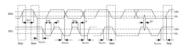
Fig 4 I<sup>2</sup>C INTERFACE TIMING
