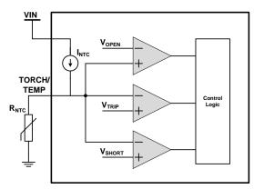
Fig 51 Temp Detection Diagram
