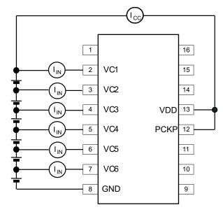
Figure 4. I<sub>CC</sub>, I<sub>IN</sub> Measurement Test Setup
