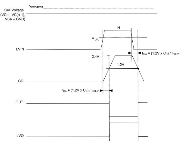
Figure 7. LVIN to OUT and LVO Timing
