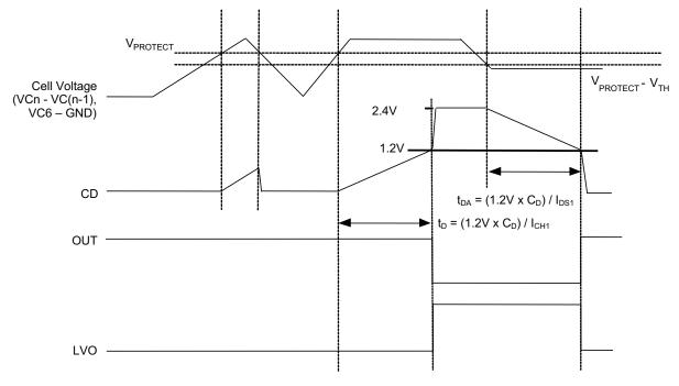
Figure 5. Timing for Overvoltage Sensing (With Recovery Option)
