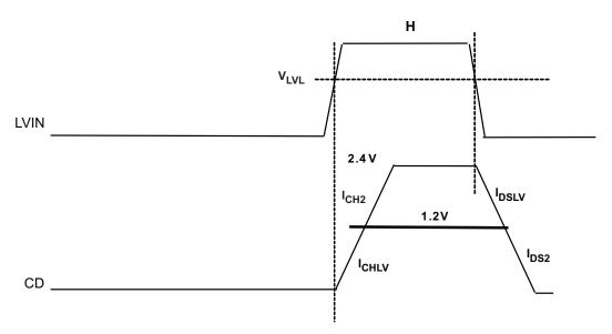
Figure 3. CD Charge Current and Discharge Current
