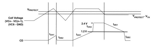
Figure 2. CD charge Current and Discharge Current
