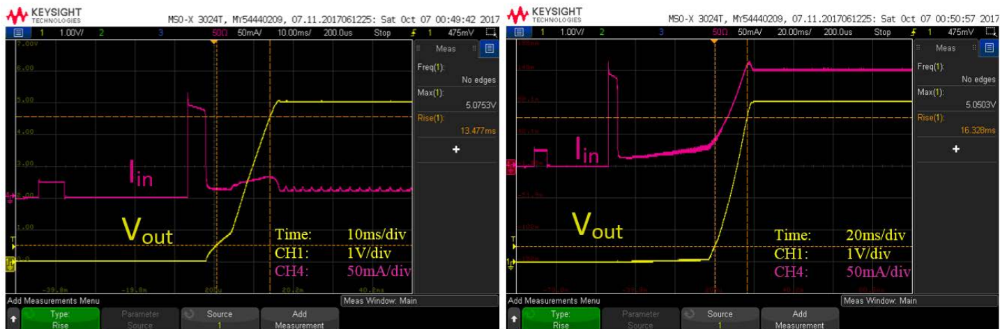
Figure 8.1. Si3404-Buck Non-Isolated EVB Output Voltage Soft-Start at Low Load (Left) and Heavy Load (Right) Conditions
