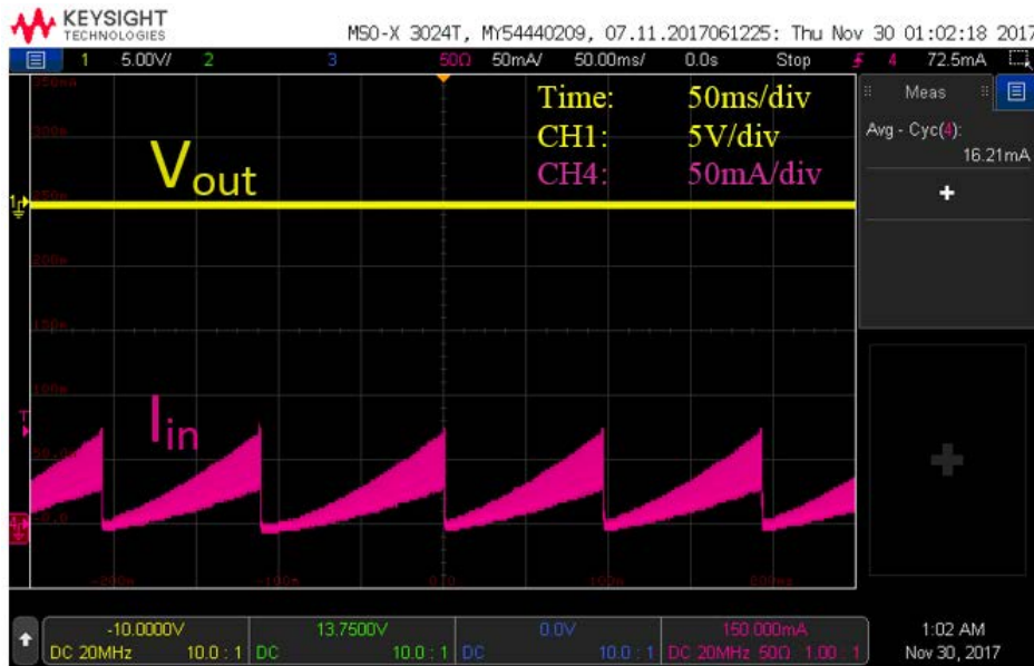
Figure 9.1. Si3404-Buck Non-Isolated EVB Output Short Circuit Protection
