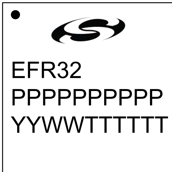
Figure 8.3. RQFN32 Package Marking
