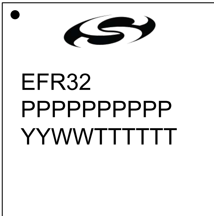
Figure 8.3. QFN48 Package Marking
