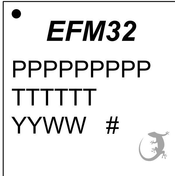
Figure 8.3. QFN32 Package Marking
