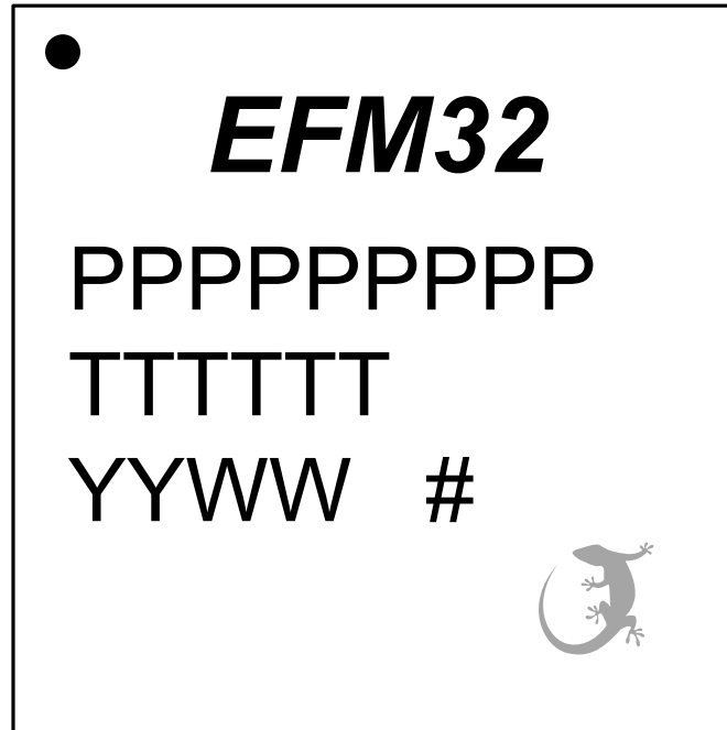
Figure 7.3. QFN48 Package Marking
