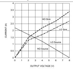
Figure 6. LO and HO Peak Gate Current vs Output Voltage **VCC = 8 V**
