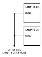
Figure 11. Sync From Multiple Devices
