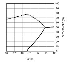
Figure 10. Mode Dependence on Duty Cycle (VOUT =12 V)
