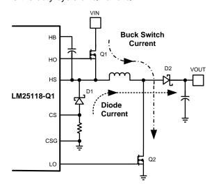
Figure 9. Buck-Boost Mode Operation
