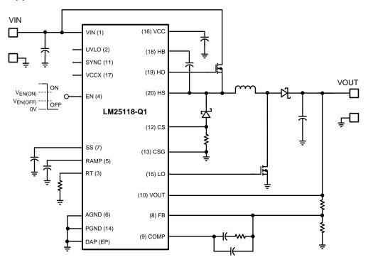
Figure 18. Typical Application Circuit
