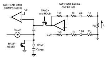
Figure 14. Current Limit and Ramp Circuit
