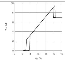
Figure 3. VCC vs VIN
