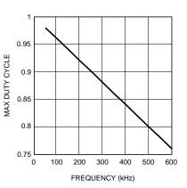
Figure 15. Maximum Duty Cycle vs Frequency
