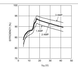
Figure 1. Efficiency vs VIN and IOUT VOUT = 12 V
