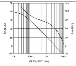
Figure 5. Error Amplifier Gain/Phase
