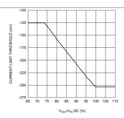
Figure 2. Current Limit Threshold vs VOUT/VIN VOUT = 12 V
