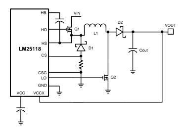
Figure 27. VCC Bias From VOUT 4 V < VOUT < 15 V
