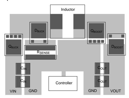
Figure 29. LM25118-Q1 Layout Example
