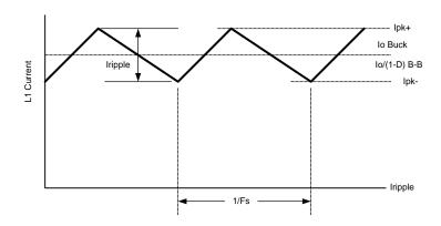
Figure 20. Inductor Current Waveform
