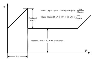
Figure 13. Composition of Emulated Current Signal
