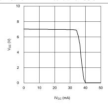
Figure 4. VCC vs IVCC
