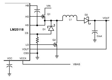
Figure 28. VCC Bias With Additional Bias Supply
