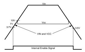
Figure 17. VIN and VCC Sequencing
