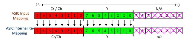
Figure 15. 16-Bit YCrCb-880 I/O Mapping
