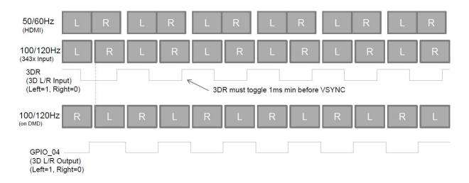
Figure 11. DLPC343x L/R Frame and Signal Timing
