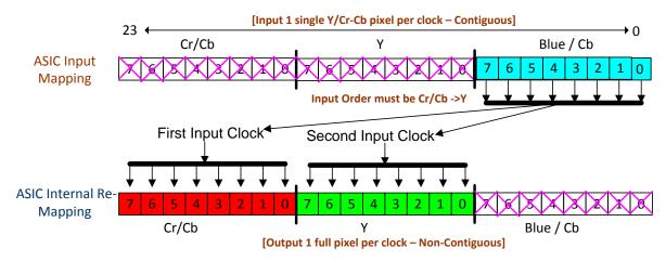
Figure 17. 8-Bit Serial YCrCb-422 I/O Mapping
