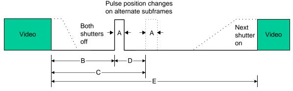
NOTE: The period between DLPLink pulses alternates between the subframe period =D and the subframe period -D, where D is the delta period.
