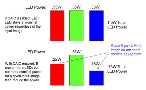
Figure 21. CAIC Power Reduction Mode (for Constant Brightness)
