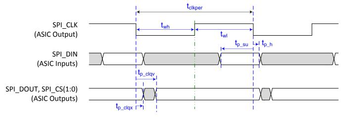
Figure 9. Flash Interface Timing
