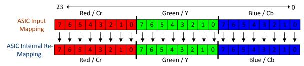
Figure 12. RGB-888 / YCrCb-888 I/O Mapping
