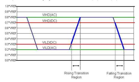
Figure 3. Low Speed (LS) I/O Input Thresholds
