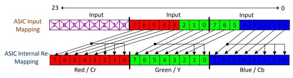
Figure 14. RGB-565 / YCrCb-565 I/O Mapping
