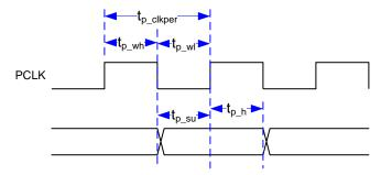
Figure 7. Parallel Interface General Timing
