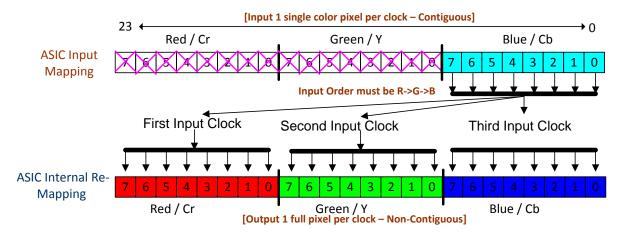
Figure 16. 8-Bit RGB-888 or YCrCb-888 I/O Mapping
