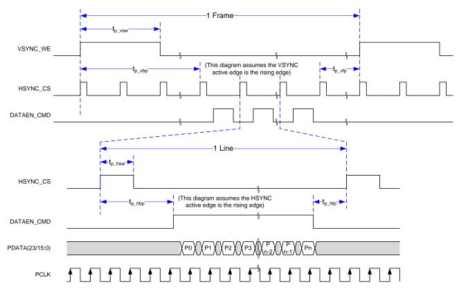
Figure 6. Parallel Interface Frame Timing
