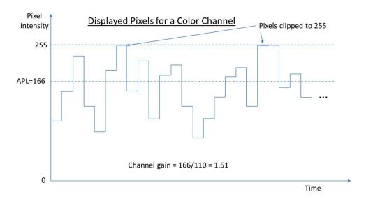
Figure 20. Displayed Pixels After CAIC Processing
