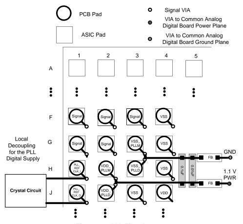
Figure 29. PLL Filter Layout
