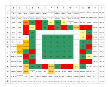
Figure 2. DLPC3438 7- x 7-mm Package – VF Ball Grid Array
