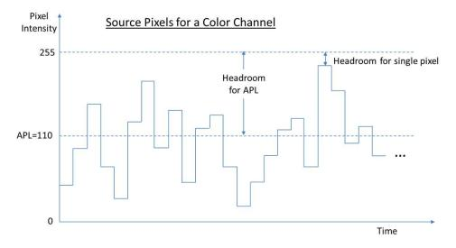
Figure 19. Input Pixels Example
