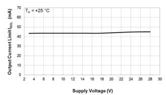
Output Current Limit vs Supply Voltage
