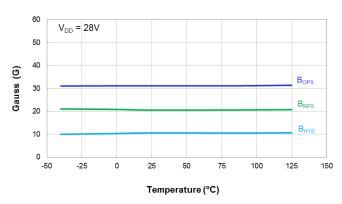
Switch Points  $\mathbf{B}_{\text{OPS}}$  and  $\mathbf{B}_{\text{RPS}}$  vs Temperature
