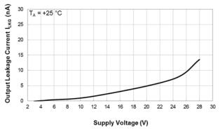
Output Leakage Current vs Supply Voltage
