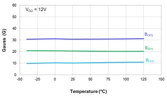
Switch Points  $\mathbf{B}_{\text{OPS}}$  and  $\mathbf{B}_{\text{RPS}}$  vs Temperature
