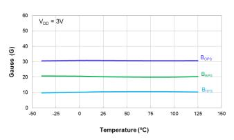
Switch Points B<sub>OPS</sub> and B<sub>RPS</sub> vs Temperature
