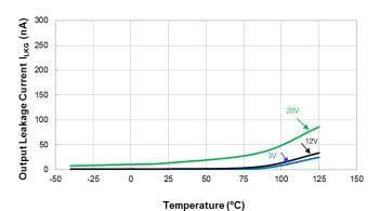
Output Leakage Current vs Temperature
