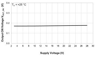
Output ON Voltage vs Supply Voltage
