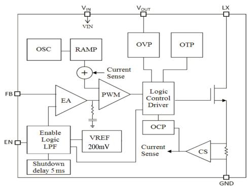
Figure 3. Simplified Block Diagram of the PT4117B
