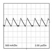
$V_{\text{IN}}$  = 12 V,  $V_{\text{O}}$  = 3.3 V,  $I_{\text{O}}$  = 0.5 A 2 µs/div
