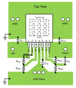
Figure 23. PCB Layout Guide
