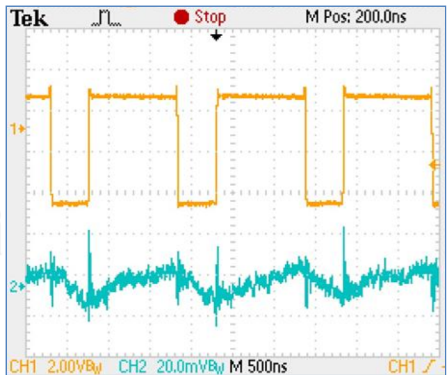
V_{IN}=3.7V, V_{OUT}=5V, I_{OUT}=1A
