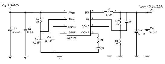
$V_{OUT} = V_{FB} x (1 + \frac{R2}{R5})$  $V_{FB} = 0.62V$ ; R5 suggest 3K ~ 6.8k
