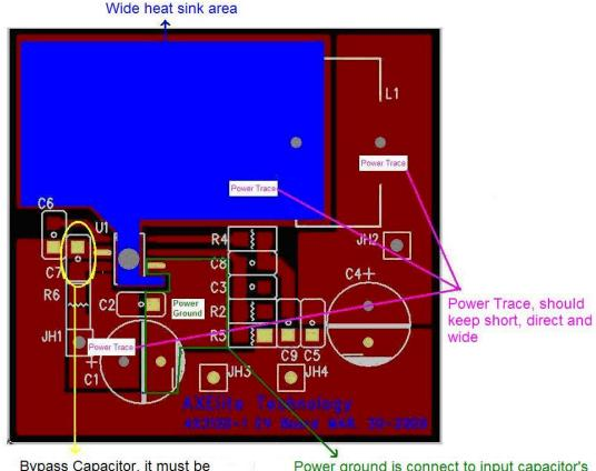
Bypass Capacitor, it must be closed to SVCC and SGND pin
