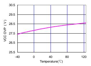
Fig. 12 VCC OVP vs. Temperature
