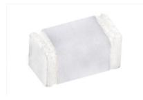
Gas discharge tubes (GDT) use noble gasses enclosed in ceramic tubes to provide an alternate circuit path for voltage spikes. The ceramic envelope and with nickel connectors allow for high loads and Ruilon offers products that function at 20KA,40KA,50KA,60KA,100KA&150KA. The breakdown voltages of the devices have a wide range (up to 20% tolerance). Major applications are high frequency telecommunication lines, stations, security systems, HID and high quality Surge Protection Devices (SPD).
