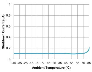
Figure 13. Shutdown Current vs. Ambient Temperature
