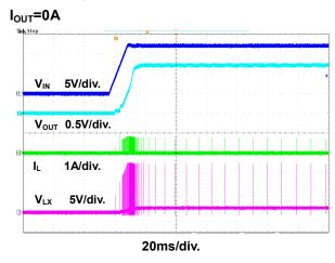
Figure 19. Startup Through Power Supply Waveform
