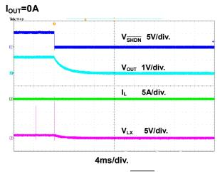
Figure 25. Shutdown Through  $\overline{\text{SHDN}}$  Waveform
