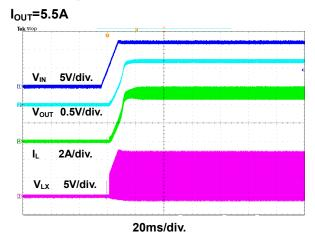
Figure 20. Startup Through Power Supply Waveform
