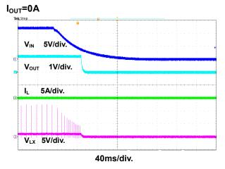
Figure 21. Shutdown Through Power Supply Waveform
