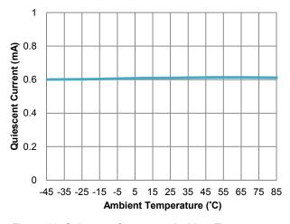
Figure 11. Quiescent Current vs. Ambient Temperature
