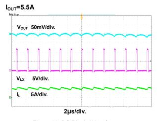
Figure 18. DC Ripple Waveform
