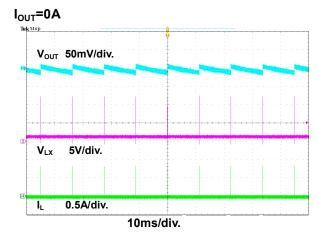
Figure 17. DC Ripple Waveform
