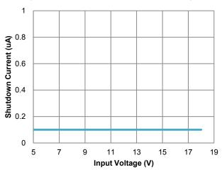
Figure 14. Shutdown Current vs. Input Voltage
