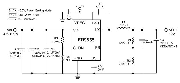
Figure 3. Application Circuit for TDFN-10 Package
