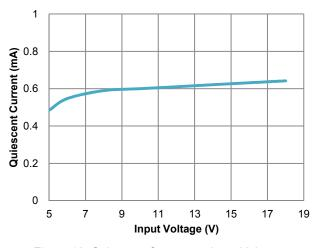
Figure 12. Quiescent Current vs. Input Voltage
