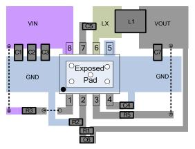
Figure 28. Recommended PCB Layout Diagram for SP Package
