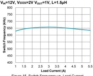
Figure 15. Switch Frequency vs. Load Current
