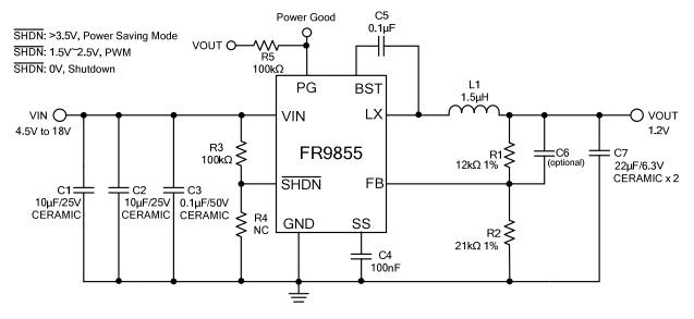
Figure 2. Application Circuit for SOP-8 Exposed Pad Package
