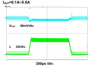
Figure 27. Load Transient Waveform
