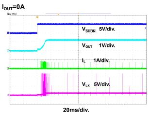
Figure 23. Startup Through SHDN Waveform
