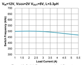
Figure 16. Switch Frequency vs. Load Current
