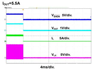
Figure 26. Shutdown Through SHDN Waveform
