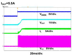
Figure 24. Startup Through SHDN Waveform
