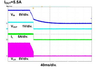
Figure 22. Shutdown Through Power Supply Waveform
