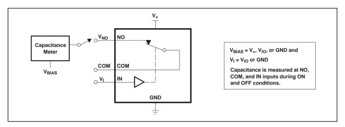
Figure 17. Capacitance (C<sub>I</sub>,  $C_{COM(OFF)}$ ,  $C_{COM(ON)}$ ,  $C_{NC(OFF)}$ ,  $C_{NC(ON)}$ )
