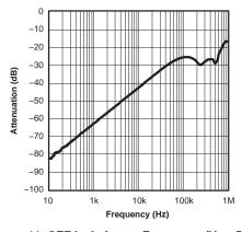
Figure 11. OFF Isolation vs Frequency  $(V_{+} = 5 V)$
