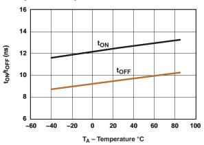
Figure 8.  $t_{ON}/t_{OFF}$  vs Temperature (V<sub>+</sub> = 5 V)
