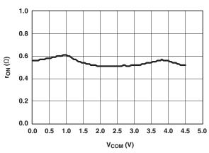
Figure 3.  $r_{on}$  vs  $V_{COM}$  ( $V_{+} = 5 V$ )
