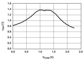
Figure 1.  $r_{on}$  vs  $V_{COM}$  ( $V_{+} = 2.5 \text{ V}$ )
