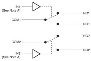
A. IN1 and IN2 are control inputs referenced to  $V_{\text{IO}}$ .
