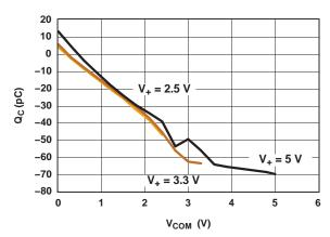
Figure 6. Charge Injection (Q<sub>C</sub>) vs V<sub>COM</sub>
