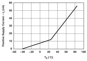
Figure 5.  $I_+$  vs Temperature ( $V_+ = 5 \text{ V}$ )
