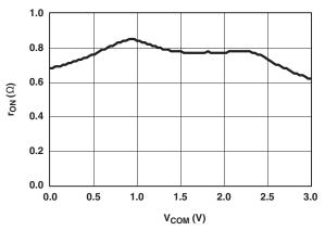
Figure 2.  $r_{on}$  vs  $V_{COM}$  ( $V_{+} = 3.3 \text{ V}$ )
