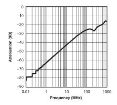
Figure 10. Crosstalk vs Frequency  $(V_+ = 5 V)$
