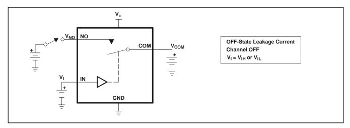
Figure 15. OFF-State Leakage Current ( $I_{COM(OFF)}$ ,  $I_{NC(OFF)}$ ,  $I_{COM(PWROFF)}$ ,  $I_{NC(PWR(FF))}$ )
