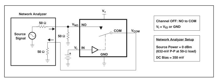
Figure 21. OFF Isolation (O<sub>ISO</sub>)
