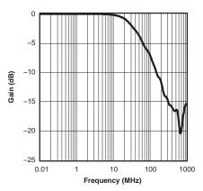
Figure 9. Gain vs Frequency  $(V_+ = 5 \text{ V})$
