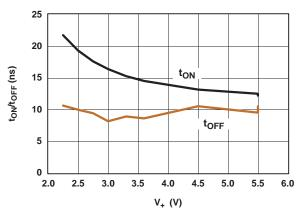
Figure 7. t<sub>ON</sub>/t<sub>OFF</sub> vs Supply Voltage
