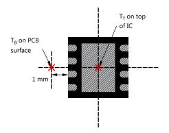
Figure 23. Measuring Points for  $T_T$  and  $T_B$
