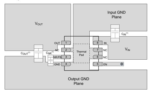
C<sub>IN</sub> and C<sub>OUT</sub> are 0603 capacitors and C<sub>NR</sub> is a 0402 capacitor. The footprint is shown to scale with package size.
