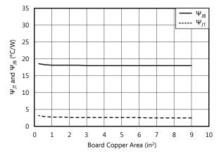
Figure 24.  $\Psi_{\text{JT}}$  and  $\Psi_{\text{JB}}$  vs Board Size
