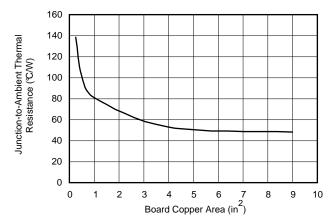
NOTE: The R<sub>0JA</sub> value at a board size of 9 in<sup>2</sup> (that is, 3 in x 3 in) is a JEDEC standard.
