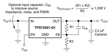
Figure 16. Typical Application Circuit for Adjustable Voltage Versions
