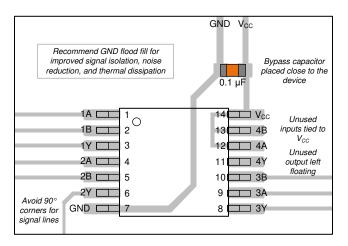
Figure 9. Example layout for the SN74HC02-Q1
