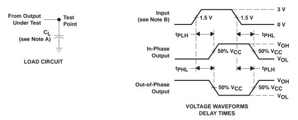
NOTES: A. C<sub>L</sub> includes probe and jig capacitance.
