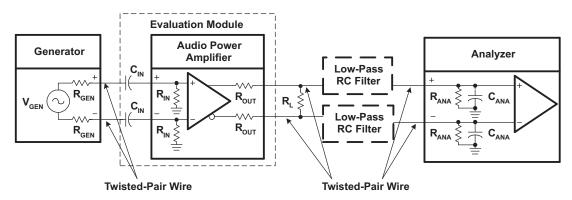
Figure 29. Differential Input, BTL Output Measurement Circuit
