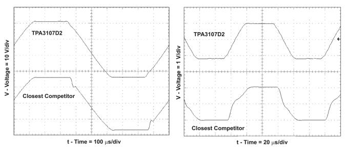
Figure 25. 1-kHz Sine Output at 10% THD+N
