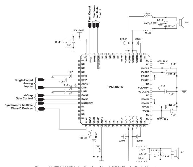
Figure 19. TPA3107D2 Application Circuit With Single-Ended Inputs
