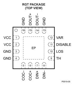
Figure 2. Pinout of ONET1191P in a 3-mm  $\times$  3-mm, 16-Pin QFN Package
