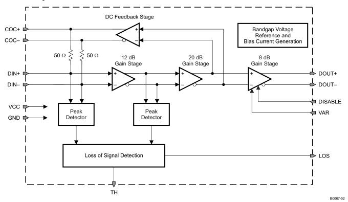
Figure 1. Simplified Block Diagram of the ONET1191P
