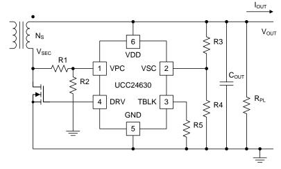
Figure 17. SR Controller Components
