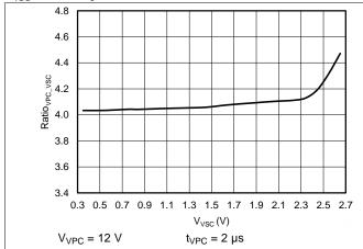
Figure 7. VPC-to-VSC Ramp-Gain Ratio vs VSC Voltage
