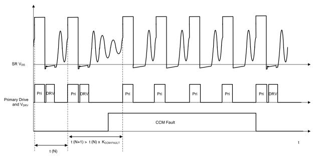
Figure 21. CCM Cycle-Fault Behavior, DCM Operation
