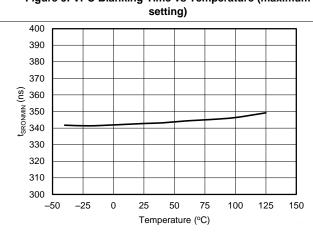
Figure 11. DRV Minimum On Time vs Temperature
