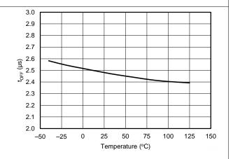
Figure 12. DRV Minimum Off Time vs Temperature
