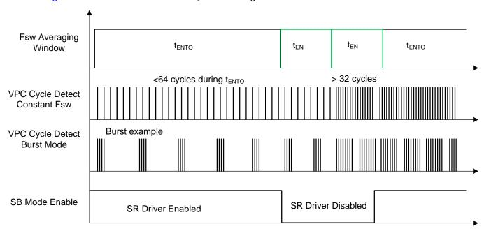
Figure 22. Standby Mode Operation
