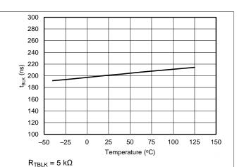
Figure 8. VPC Blanking Time vs Temperature (minimum setting)
