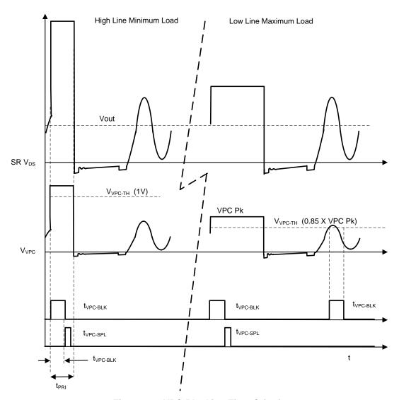
Figure 18. VPC Blanking Time Criteria
