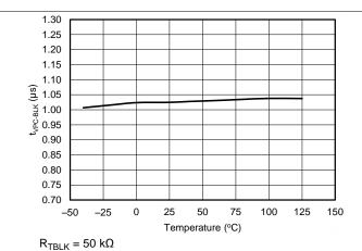
Figure 9. VPC Blanking Time vs Temperature (maximum
