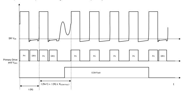
Figure 20. CCM Cycle-Fault Behavior, CCM Operation
