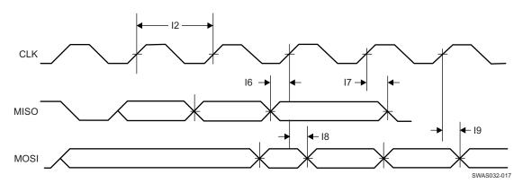
Figure 4-14. Flash SPI Interface Timing
