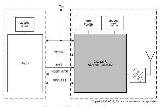
Figure 5-1. Functional Block Diagram
