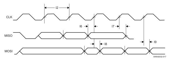
Figure 4-13. Host SPI Interface Timing
