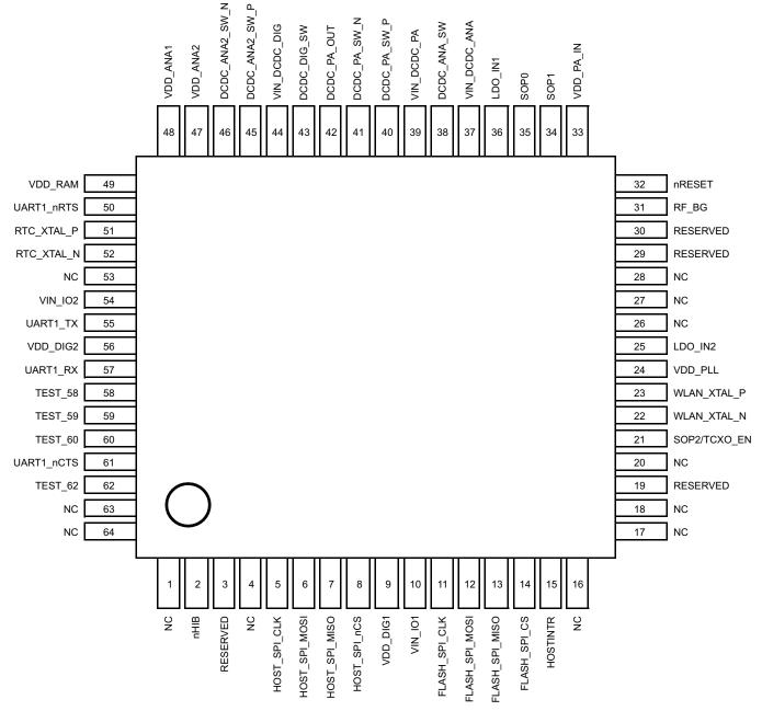
Figure 3-1. VQFN 64-Pin Assignments Top View
