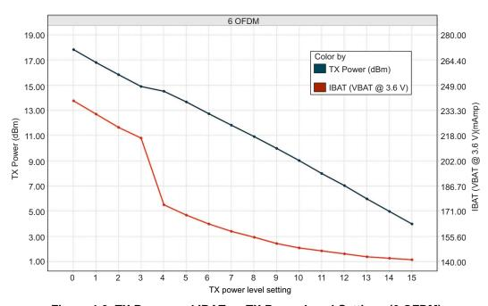
Figure 4-2. TX Power and IBAT vs TX Power Level Settings (6 OFDM)
