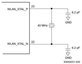
NOTE: The XTAL capacitance must be tuned to ensure that the PPM requirement is met. See CC31xx & CC32xx Frequency Tuning for information on frequency tuning.
