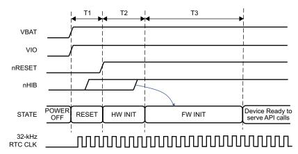
Figure 4-7. First-Time Power-Up and Reset Removal Timing Diagram (External 32K)
