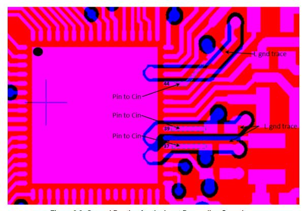
Figure 6-3. Ground Routing for the Input Decoupling Capacitors
