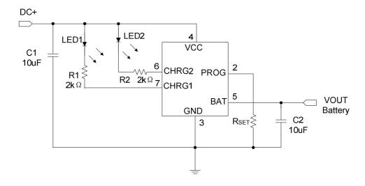
Figure 1: Typical Application Circuit with Two LEDs
