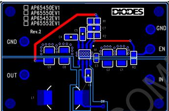
Figure 7 PC Board Layout for SO-8EP
