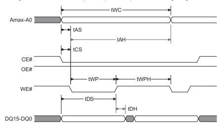
Figure 21. Back to Back (CE#VIL) Write Operation Timing Diagram<sup>[154]</sup>
