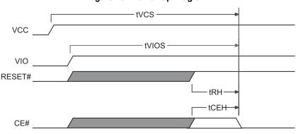
Figure 15. Power-Up Diagram
