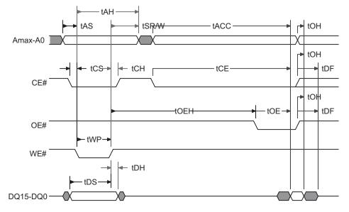
Figure 23. Write to Read (t<sub>CE</sub>) Operation Timing Diagram<sup>[155]</sup>
