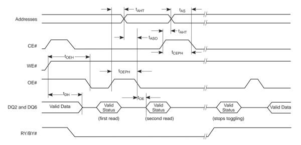
Figure 30. Toggle Bit Timing Diagram (During Embedded Algorithms)<sup>[165]</sup>
