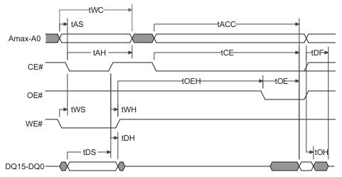
Figure 33. (CE#) Write to Read Operation Timing Diagram<sup>[169]</sup>
