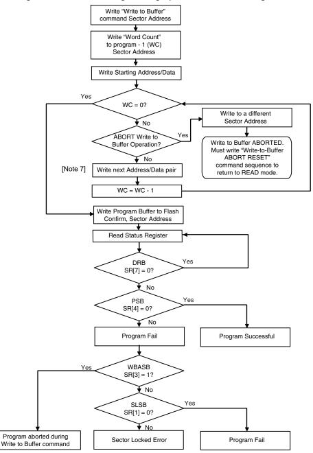
Figure 5. Write Buffer Programming Operation with Status Register
