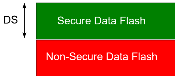
Figure 13-3. SAM L11 Data Flash Memory Mapping
