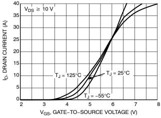
Figure 2. Transfer Characteristics
