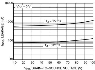
Figure 6. Drain-to-Source Leakage Current versus Voltage
