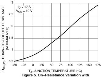
Figure 5. On–Resistance Variation with Temperature
