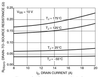
Figure 4. On-Resistance versus Drain Current and Gate Voltage
