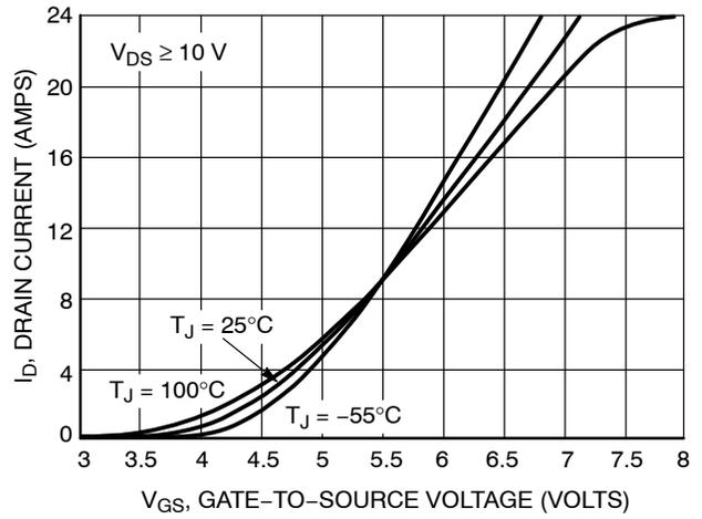
Figure 2. Transfer Characteristics
