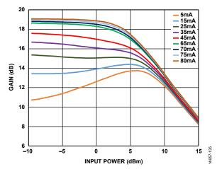
Figure 36. Gain vs. Input Power for Various Supply Currents (IDQ) at 5 GHz,  $V_{\rm DD}$  = 5 V
