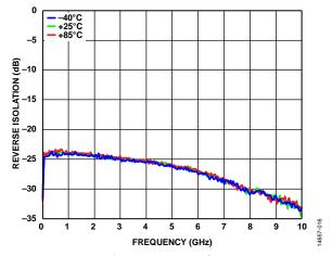
Figure 17. Reverse Isolation vs. Frequency for Various Temperatures
