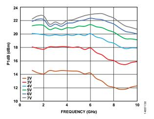
Figure 31. P1dB vs. Frequency for Various Supply Voltages,  $I_{DQ} = 65 \text{ mA}$
