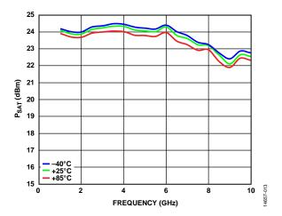
Figure 13. P<sub>SAT</sub> vs. Frequency for Various Temperatures
