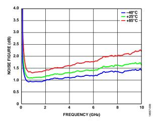
Figure 8. Noise Figure vs. Frequency for Various Temperatures
