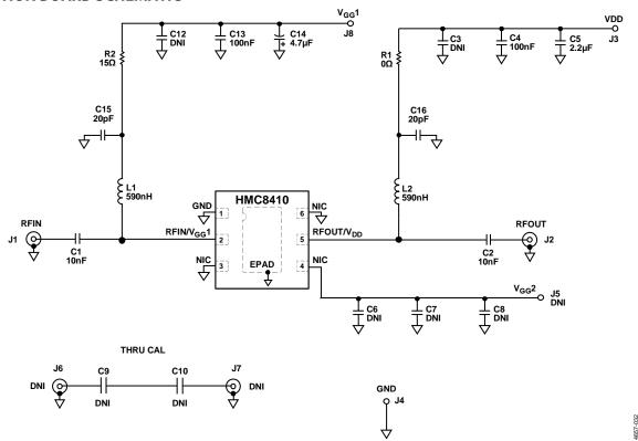
Figure 41. HMC8410 Evaluation Board Schematic
