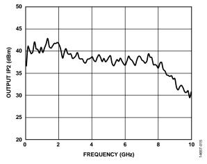
Figure 15. Output IP2 vs. Frequency at Pout/Tone = 5 dBm
