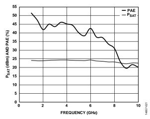
Figure 22. Psat and PAE vs. Frequency
