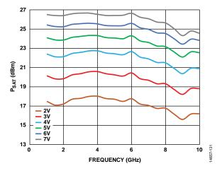
Figure 32.  $P_{SAT}$  vs. Frequency for Various Supply Voltages,  $I_{DQ} = 65 \text{ mA}$
