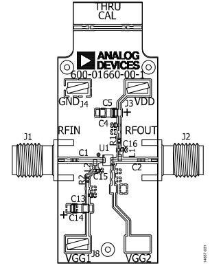
Figure 40. HMC8410 Evaluation PCB
