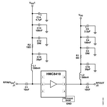
Figure 39. Typical Application Circuit
