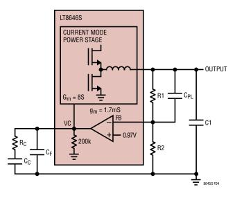
Figure 4. Model for Loop Response
