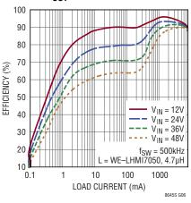
LT8646S Low Load Efficiency at 3.3V<sub>OUT</sub>
