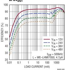
LT8646S Low Load Efficiency at 5V<sub>OUT</sub>
