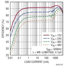
LT8645S Low Load Efficiency at 5V<sub>OUT</sub>
