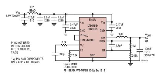
Figure 10. Ultralow EMI 5V, 8A Step-Down Converter with Spread Spectrum
