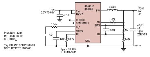
Figure 8. 5V 8A Step-Down Converter with Soft-Start and Power Good
