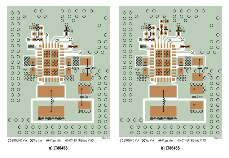
Figure 1. Recommended PCB Layouts for the LT8645S and LT8646S
