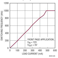
Minimum Load to Full Frequency (Pulse-Skipping Mode)
