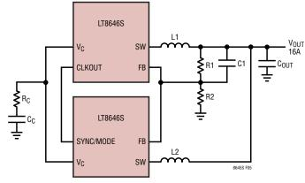
Figure 5. Paralleling Two LT8646S
