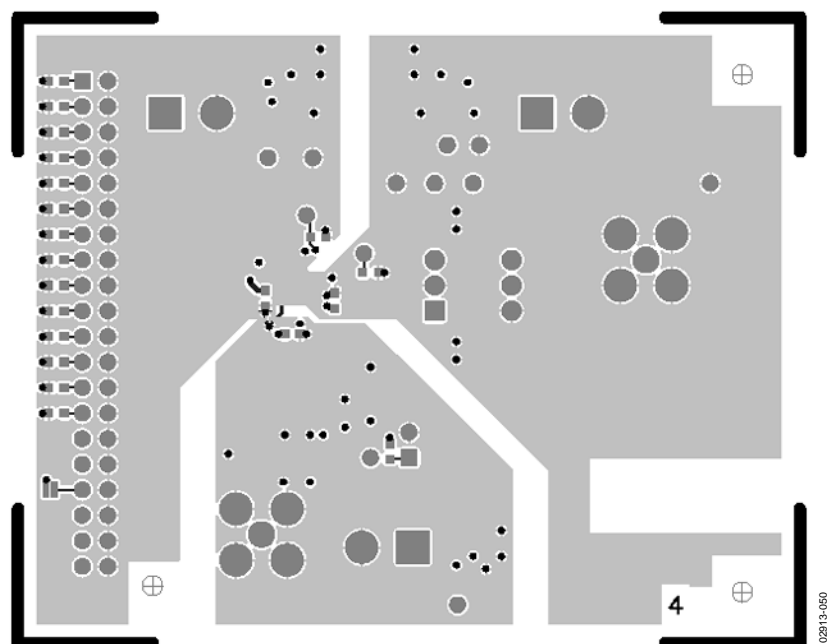
Figure 53. LFCSP Evaluation Board Layout—Secondary Side
