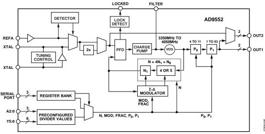
Figure 19. Detailed Block Diagram
