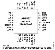
Figure 2. Pin Configuration
