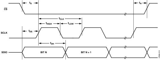
Figure 29. Serial Control Port Timing—Write
