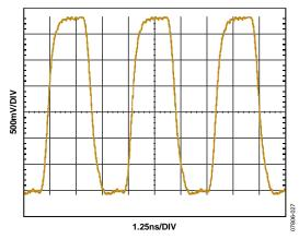
Figure 16. Typical Output Waveform, CMOS (250 MHz, 15 pF Load)
