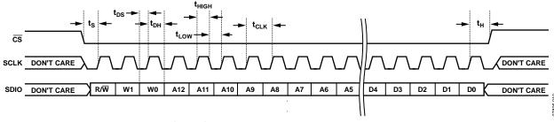
Figure 26. Serial Control Port Write—MSB First, 16-Bit Instruction, Timing Measurements
