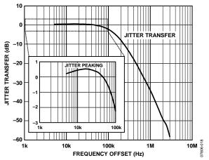
Figure 5. Jitter Transfer and Jitter Peaking
