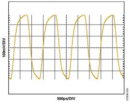
Figure 15. Typical Output Waveform, LVDS (805 MHz, 3.5 mA Drive Current)
