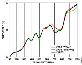
Figure 13. Duty Cycle vs. Output Frequency, LVPECL and LVDS (15 pF Load)
