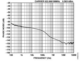
Figure 6. Phase Noise, Integer, SDM Off  $(f_{XTAL} = 19.44 \text{ MHz}, f_{OUT1} = 622.08 \text{ MHz})$
