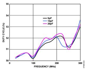
Figure 11. Duty Cycle vs. Output Frequency, CMOS
