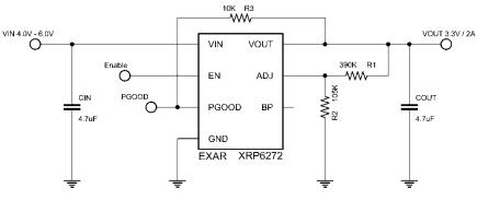
Fig. 23: 5V to 3.3V / 2A
