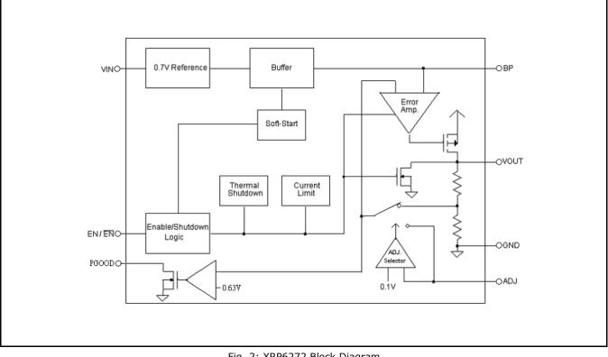
Fig. 2: XRP6272 Block Diagram
