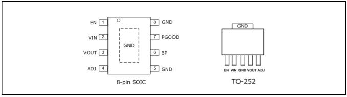
Fig. 3: XRP6272 Pin Assignment
