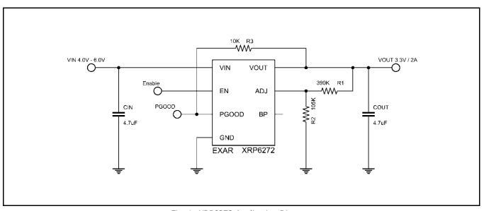
Fig. 1: XRP6272 Application Diagram
