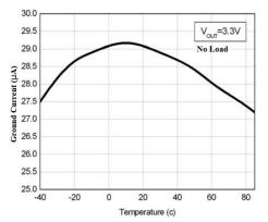
Fig. 9: GND Current vs. Temp. at VOUT=3.3V, No Load
