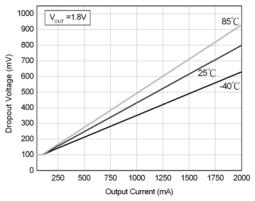
Fig. 10: Dropout Voltage at VOUT = 1.8V
