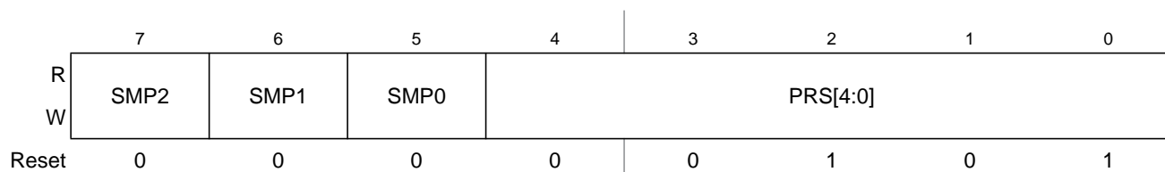
Figure 10-8. ATD Control Register 4 (ATDCTL4)
