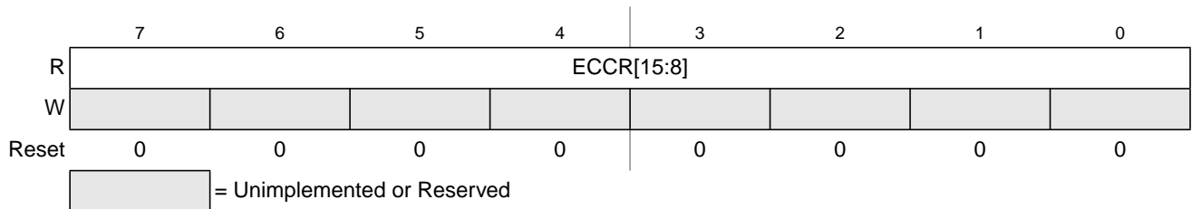
Figure 18-20. Flash ECC Error Results High Register (FECCRHI)
