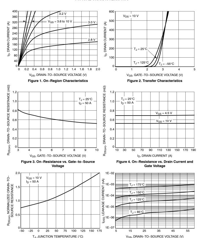
Figure 5. On–Resistance Variation with Temperature
