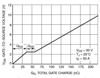
Figure 8. Gate-to-Source Voltage vs. Total Charge
