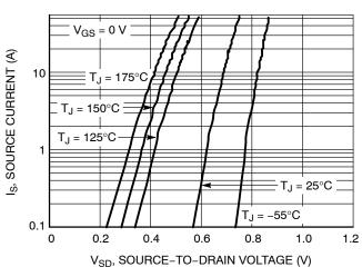
Figure 10. Diode Forward Voltage vs. Current
